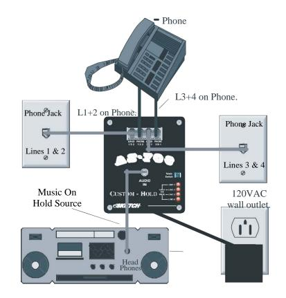
When a line is placed "ON HOLD", the corresponding LED on the AS-703- H will light indicating that music on hold audio is being coupled to that telephone line. The unit will play music on hold audio to all calls that are placed ON HOLD. Make sure that you adjust the level of the music on hold to the proper level on the music on hold source.
