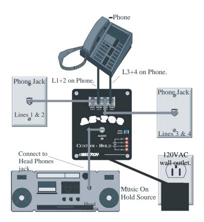
When a line is placed "ON HOLD", the corresponding LED on the AS- 703-M will light indicating that music on hold audio is being coupled to that telephone line. The unit will play music on hold audio to all calls that are placed ON HOLD. Make sure that you adjust the level of the music on hold to the proper level on the music on hold audio source.
