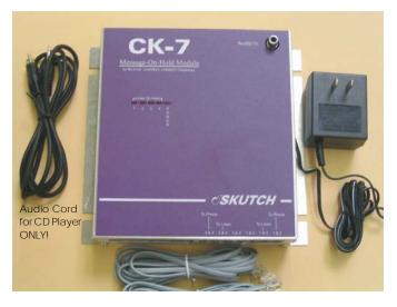
any one of the compatible telephones and is accessible from all compatible telephones that are connected to the same telephone lines. Other makes and/or models of telephones can be used with the CK-7 but they will not produce music on hold audio when placed ON HOLD.
