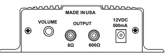
VOLUME - This pot is used to control the  $8\Omega$  and  $600\Omega$  output level of the music on hold messages. Volume up is clockwise, volume down is counter-clockwise.
