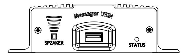
SPEAKER - The SPEAKER switch can be turned ON and OFF to monitor music on hold audio playback. The switch has no effect on the audio output connections on the rear of the unit. Switch should normally be kept OFF.
